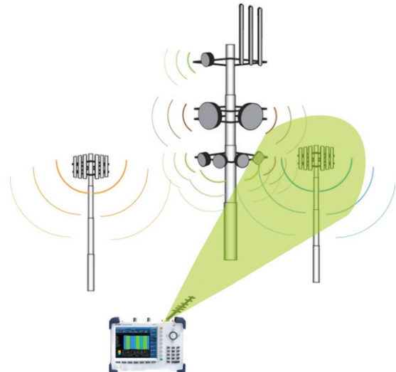
Fig 15. Interference Location with Directional Antenna
