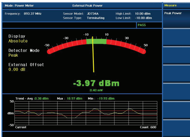
Power meter test (RF or optical)
