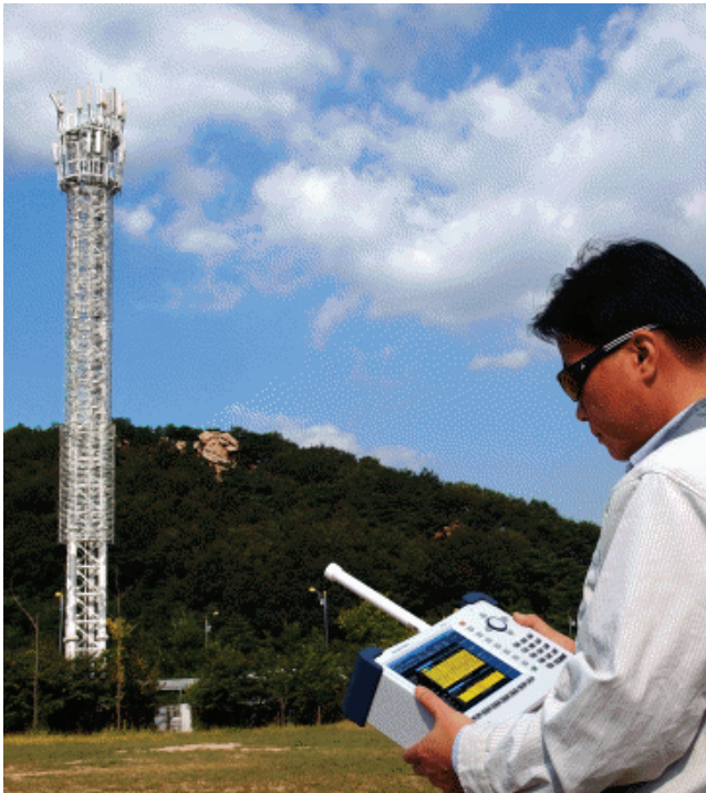
The outdoor display mode enables easier reading in direct sunlight
