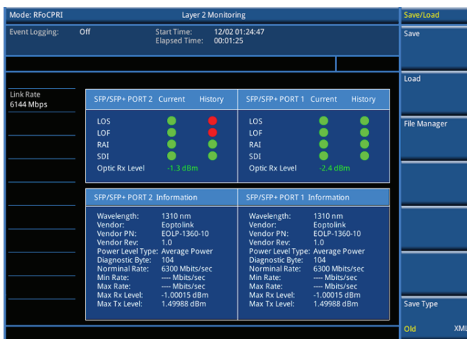
RFoCPRI — Layer-2 Monitoring
