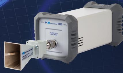
DR-01 Installed on EMI Receiver model 9180
