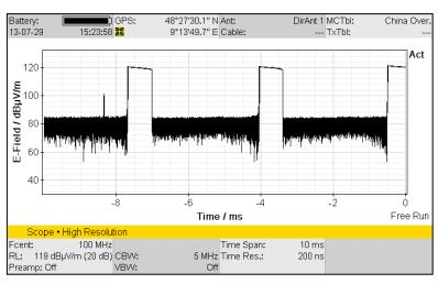
Direct examination of the defective device. Scope mode shows the time characteristic of the interference signal level exactly.
