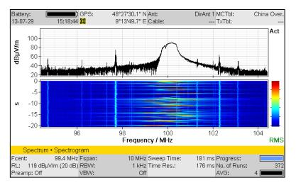
A single spectrum (above) taken from the spectrogram (below). The time characteristic can be followed by retrieving the individual spectrums one after the other.
