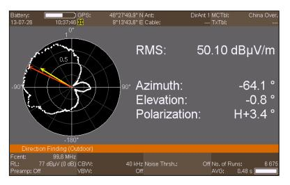
A Horizontal Scan, i.e. taking bearings all round, at a frequency of 99.6 MHz and a bandwidth of 40 kHz. The result is shown as a polar diagram. The red arrow indicates the maximum and hence the suspected direction of the interference source.
