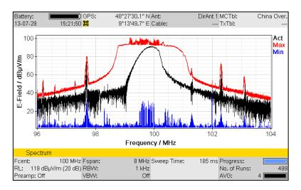
Spectrum mode. The type of interference becomes clear when you display the actual, maximum and minimum levels.
