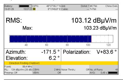
The final meters of direction finding: Looking for the maximum level.
