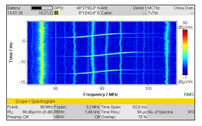
A gapless spectrogram covering 15 ms. The interference appears roughly every 3.8 ms and takes about 0.8 ms to move from a lower to a higher frequency across a variable bandwidth.
