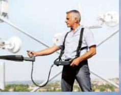
The overmodulation resistance of the preamplifier means that it is possible to insert a filter between it and the basic unit. The IDA 2 can store all the relevant transfer factors in the signal chain, from the antenna conversion factor to the preamplifier, filter, external attenuators and RF cable, and takes them into account together with the transfer function of its input stage when displaying the results.
