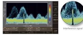
The Persistence view shows the incidence of a particular amplitude value at a given frequency in different colors. This makes it easy to spot sporadic signals. Interference that in other views is swamped by the wanted signal can be easily distinguished because of the color differences.
