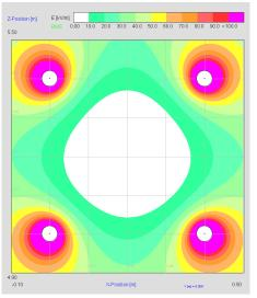
Fig. 6. Four-conductor bundle surface field strength
