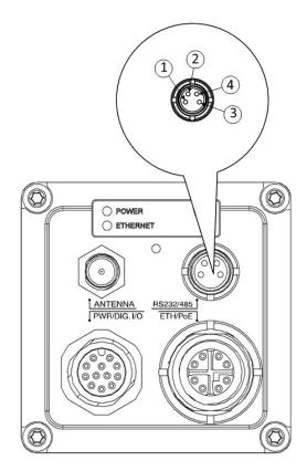
Figure 11.5 Male A-coded M8 RS232/RS485 connector
