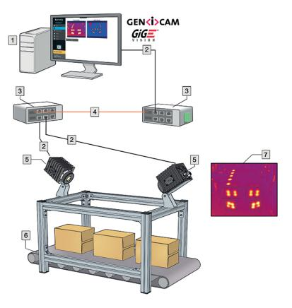
Figure 5.2 Checking hot glue on cardboard boxes
