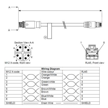
Figure 11.2 Ethernet cable M12 to RJ45
