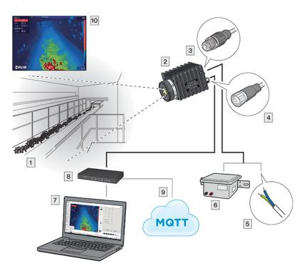
Figure 5.1 Hot spot detection, self-combustible material on conveyor belt
