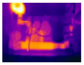
MSX (Multi Spectral Dynamic Imaging): The camera displays the thermal image where details from the visual image have been added.
