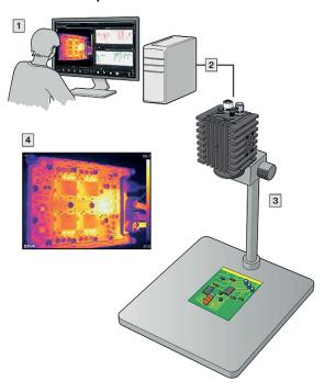
Figure 5.4 Checking heat dissipation on PCB during development
