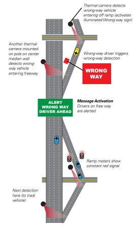
A dynamic incident detection system allows traffic authorities to detect wrong-way drivers very fast, right at the highway's entry point.
