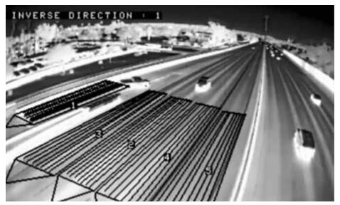
Thermal imaging cameras pick up heat coming off the environment and are therefore the ideal tool to detect vehicles on highways or on highway ramps.
