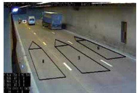
FLIR ITS-Series Dual AID cameras combine thermal and visual imaging with video analytics to provide a complete automatic incident detection solution.
