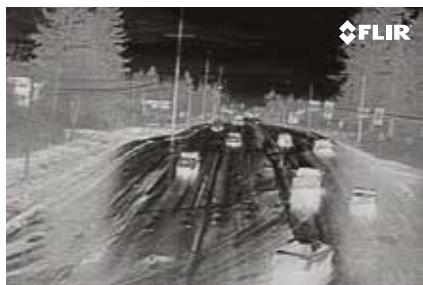
Daylight image and thermal image of an intersection. Note that the thermal images show much more detail, even when the sun is shining on the wet road.
