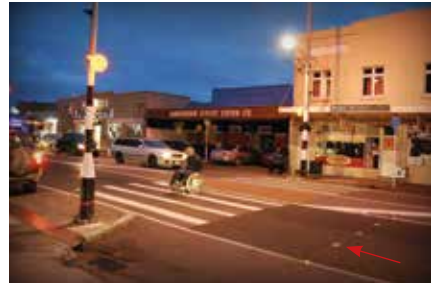
FLIR's C-Walk and SafeWalk video sensors activate on-road markers along a zebra crossing when a pedestrian is in range.
