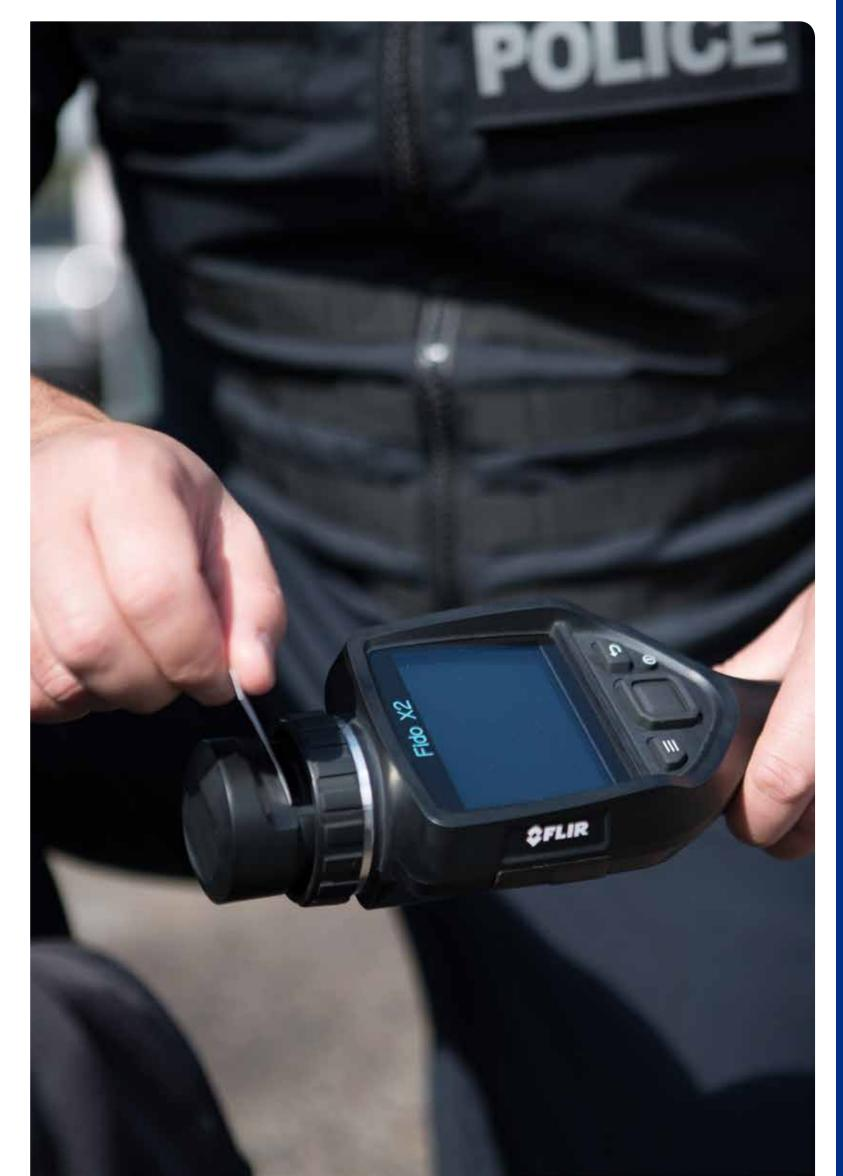
ETD in its class. Its unique TrueTrace™ detection technology identifies military, conventional, homemade, and liquid explosive threats by class on surfaces (particulate) and in bottles (vapor). With a magnesium case and splash-proof seal, its rugged design meets rigorous MIL-STD-810G and IP54 specifications.
