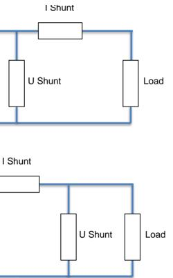
Measurement on low current loads If measuring low current loads, the primary accuracy is laid on the current. In this case we measure the true current trough the load and take into account that we will have an influence on the accuracy on the voltage measurement, caused by the additional small voltage drop over the current shunt (I Shunt)
